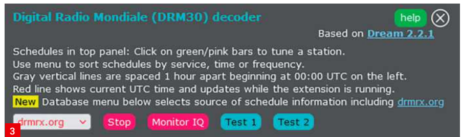
Fig. 2: The DRM Extension launches the Decoder and the Schedule windows. Clicking on a schedule entry configures the SDR automatically.
